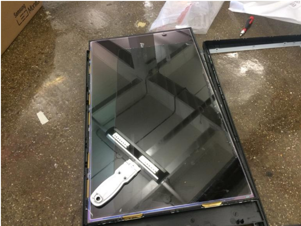
Image of attempting to slowly scrape the film off of a monitor with a razor blade
